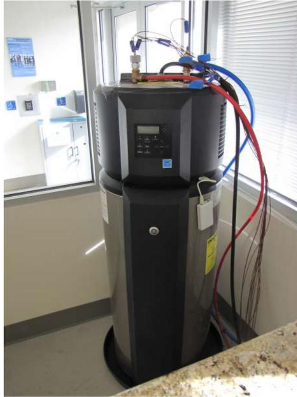
**Figure 3. Residential water heaters are a flexible load that can provide a range of grid services—including load shifting and frequency regulation—without impacting occupants. This GE heat pump water heater is shown being tested at NREL’s Advanced Home Energy Management Laboratory. Image courtesy of NREL.**
